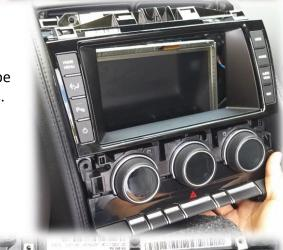
9. Remove (4x) Torx t20 screws securing the screen. Disconnect all associated harnesses and set the screen aside in a safe place.
