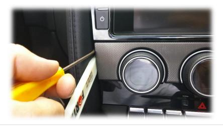
7. Remove (2x) Torx t20 screws beneath this panel (not shown).
