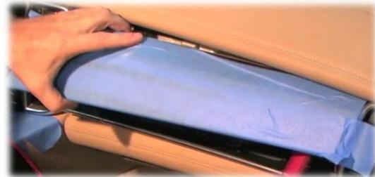
2. **Driver's side;** Insert pry tool into the bottom of the panel between the steering column and AC vent, gently pry. Disconnect the wiring, set panel aside.
